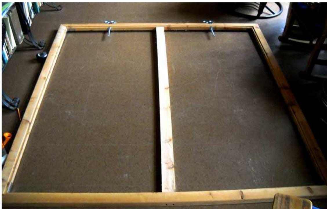
This is the frame for the middle window, measuring roughly 78 inches tall and 72 inches wide. You can see that we ripped a 1/2-inch wide, 1/4-inch deep trough into the inside edges of the frames, on the inside of the panel, to hold the Reflectix in place without compressing it. The Reflectix was then cut and taped into place using aluminum foil tape. You can see the result below on one of the narrow shutters.
