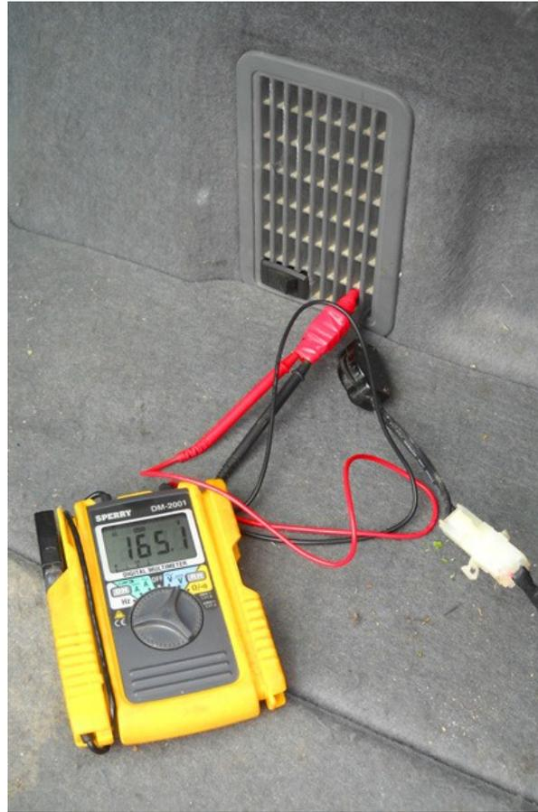
I simply carved a space for a high-voltage rocker switch in the plastic vent cover and routed the 12-volt fan cord (line switch and white connector) and traction battery monitor cord (red) through the vent face. The meter shows a resting voltage (no charge or discharge) of 165.1 volts DC.
